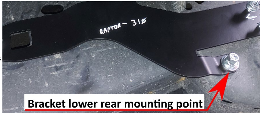
Figure 35- Rear Horn Bracket Fastened
