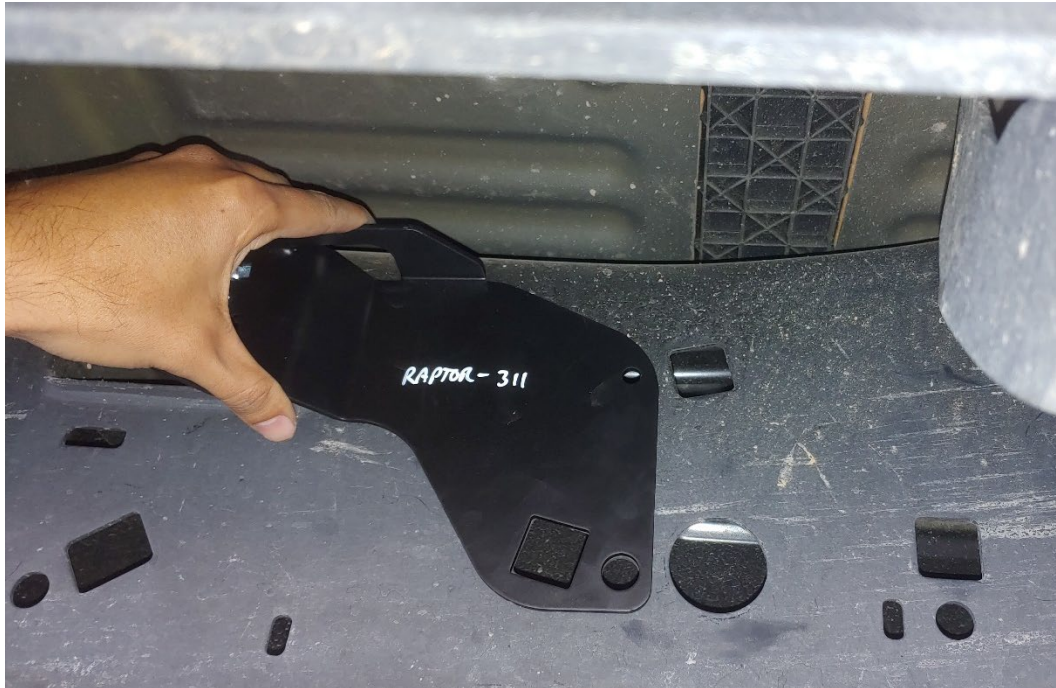
Figure 24- Installation Orientation of the Front Horn Bracket
