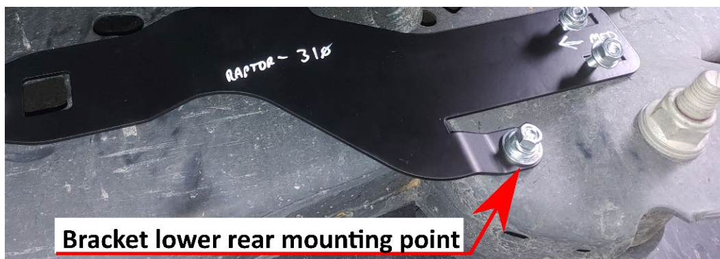
Figure 30- RAPTOR-310 Lower Mounting Point Installed
