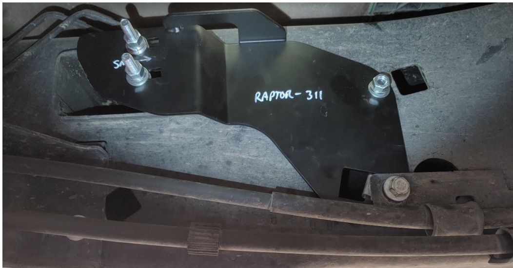
Figure 27- Front Horn Bracket Installed
