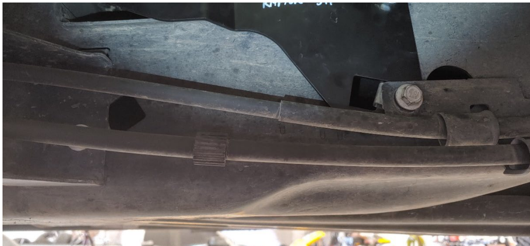
Figure 25- Bracket Fastened to Lower Mounting Point
