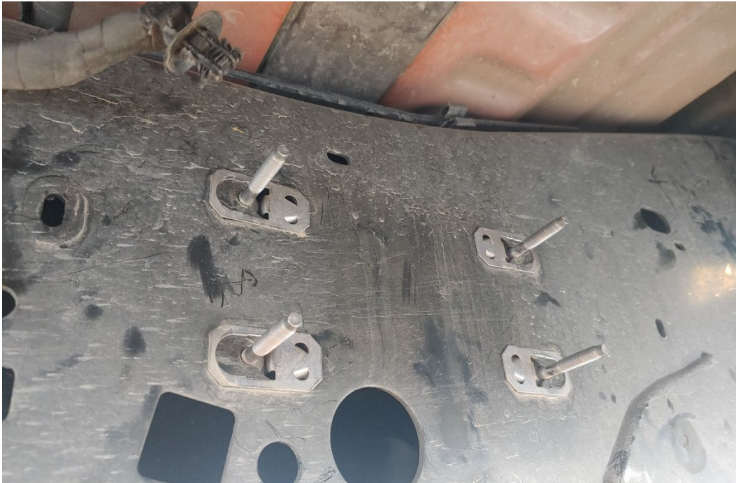
Figure 33- Module & Wire Harness Removed
