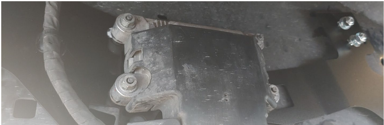
Figure 37- Module & Horn Brackets Fully Installed
