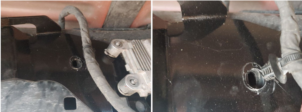
Figure 36- Wire Bundle Re-Attached
