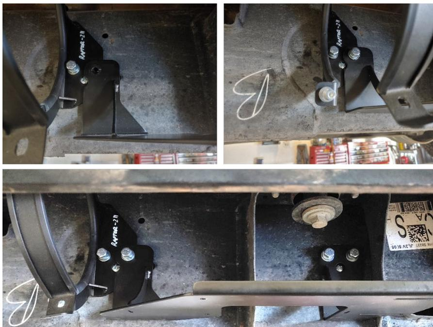
Figure 9- Compressor & Front Tank Bracket Installed
