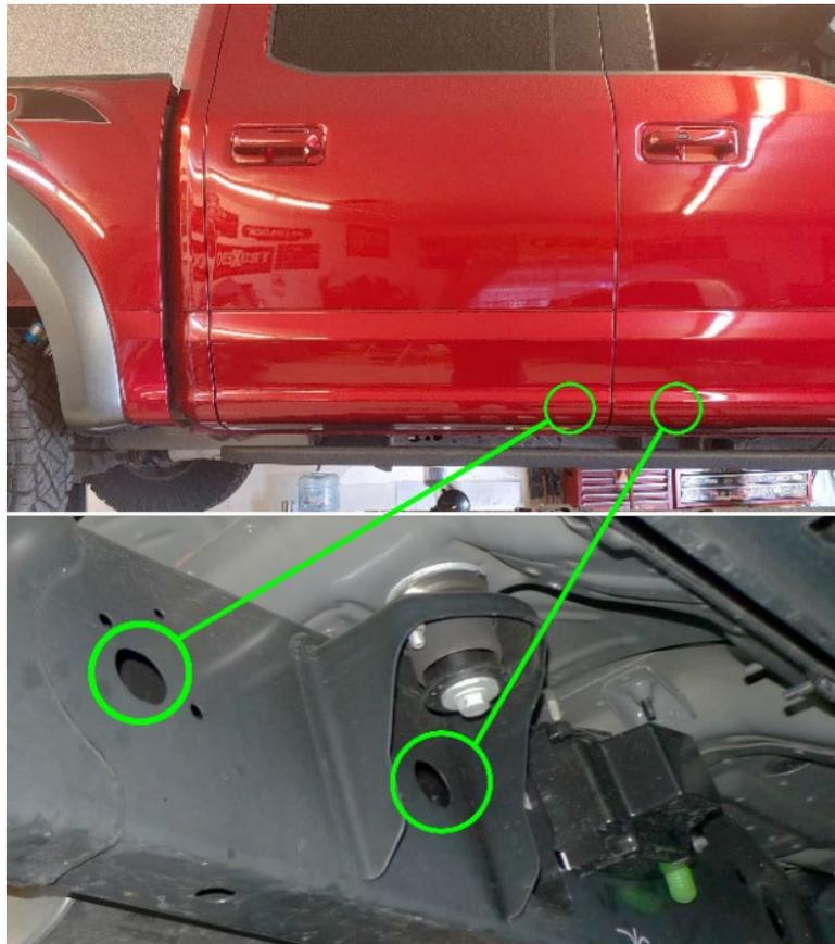
Figure 6- Nut Plates (RAPTOR-203) Install Locations
