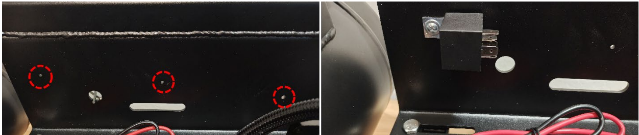
Figure 22- Relay Installation - USTL Bracket Option
