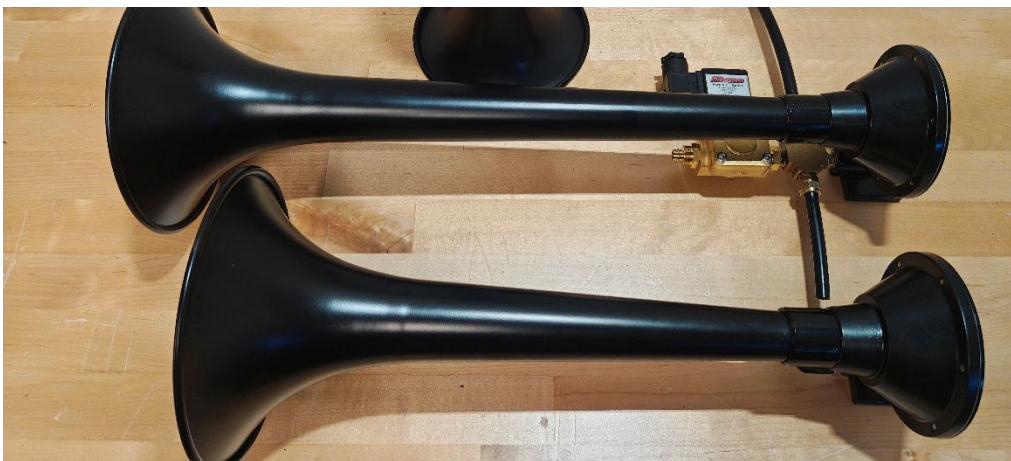
Figure 13- Horns Reassembled & Ready for Install
